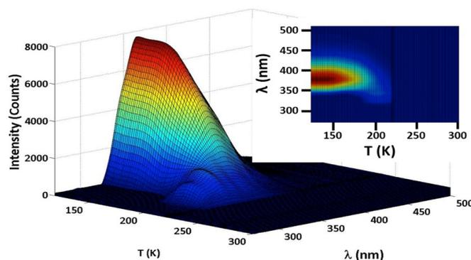
**Figure 4.** Wavelength resolved TPD of multilayer biphenyl with  $\Theta_{\text{biphenyl}} \sim 250$  ML but spectrum at 220 K subtracted from Figure 3 so that only the excimer is apparent. Inset is the top view.
