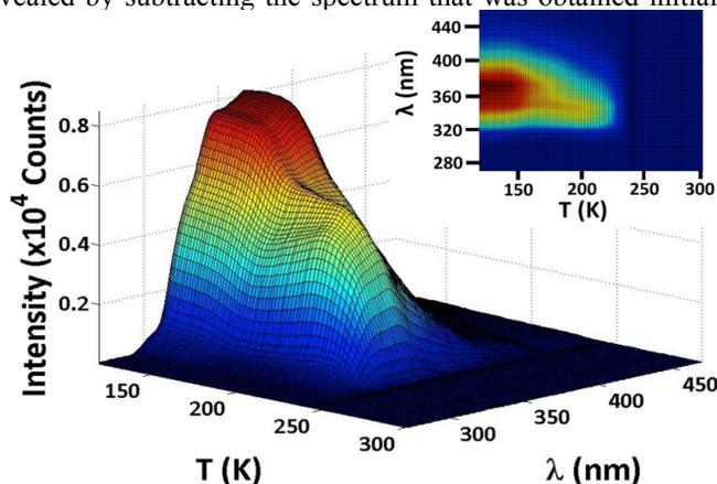
**Figure 3.** Wavelength resolved TPD of multilayer biphenyl with  $\Theta_{\text{biphenyl}} \sim 116$  ML. Deposition temperature = 135 K. The intensity of the excimer with  $\lambda_{\text{max}}$  at 370 nm dominate. The planar ordered biphenyl at 345 nm is also visible. Inset is the top view.
