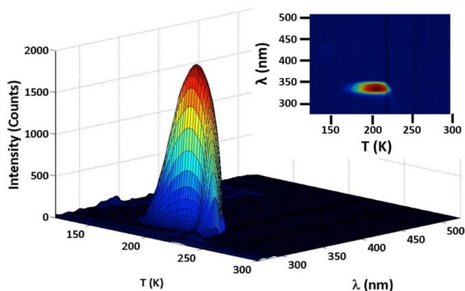
**Figure 5.** Wavelength resolved TPD of multilayer biphenyl with  $\Theta_{\text{biphenyl}} \sim 167$  ML but spectrum at 110 K subtracted from Figure 3 so that only the ordered planar conformer of biphenyl is observed. Inset is the top view.
