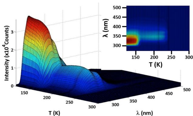
**Figure 1.** Wavelength-resolved TPD of multilayer biphenyl with  $\Theta_{\text{biphenyl}} \sim 384$  ML. Initially the amorphous twisted conformer is observed with  $\lambda_{\text{max}} \sim 320$ . At the transition temperature at  $161 \pm 1$  K the intensity decreases to  $\sim 20\%$  and the  $\lambda_{\text{max}}$  red shifts to  $\sim 345$  nm which is the ordered planar conformer. Inset is the top view.
