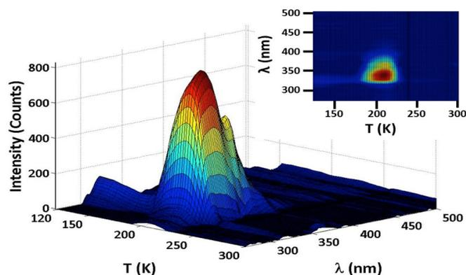
**Figure 9.** Wavelength resolved TPD of multilayer biphenyl with  $\Theta_{\text{biphenyl}} \sim 50$  ML with the absence of the excimer fluorescence intensity.
