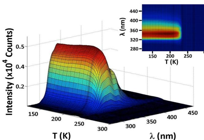
**Figure 2.** Wavelength-resolved TPD of multilayer biphenyl with  $\Theta_{\text{biphenyl}} \sim 91$  ML. Deposition temperature = 165 K. Only the ordered planar conformer of biphenyl is observed. Inset is the top view.
