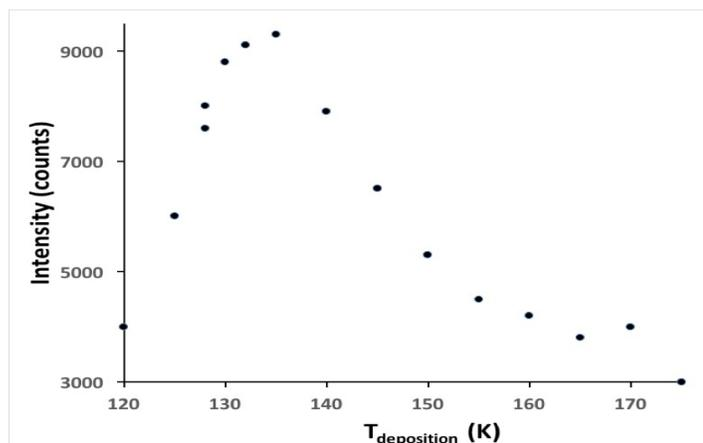
**Figure 6.** Plot of the intensity of the excimer at 370 nm as a function of deposition temperature.  $\Theta_{\text{biphenyl}}$  was held at  $120 \pm 20$  ML.
