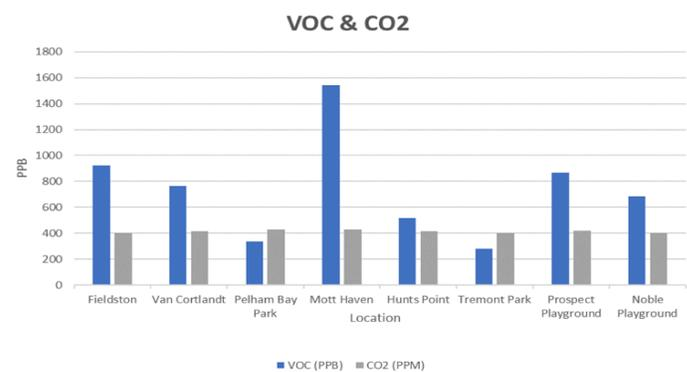
Figure 5: VOC & CO<sub>2</sub> Measurements
