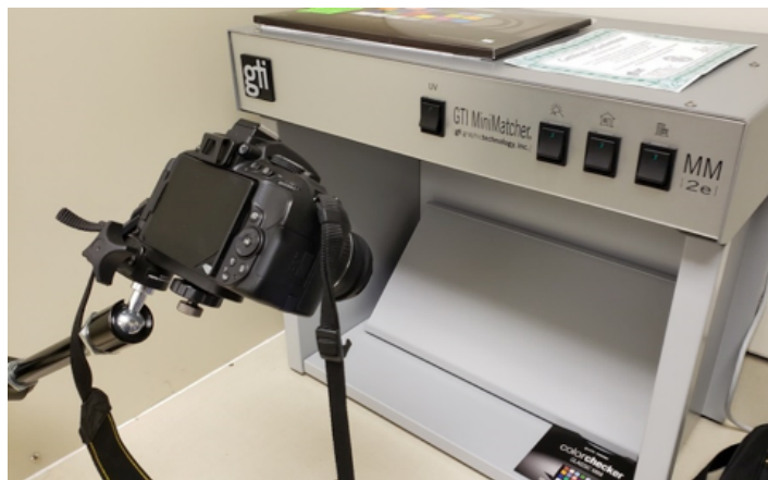
Figure 3. Yellowness index color test setup
