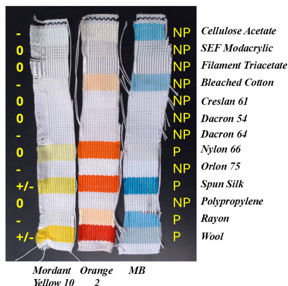
Figure 2. Multi-fabric test strips stained with three of the dyes used in this work (strips stained with orange 1 were very similar to those stained with orange 2). The charge on the fabric polymer, positive (+), negative (-), neutral (0), or zwitterionic (+/-) is indicated on the left in yellow, while the polarity is indicated on the right in yellow. The protein fabrics (silk and wool) bound all types of dye well. The polymers that stained best with anionic diazo dyes were nylon 6,6 and to a lesser extent, cotton and rayon. The polymers that bound MB selectively were negatively charged including cellulose acetate and rayon.
