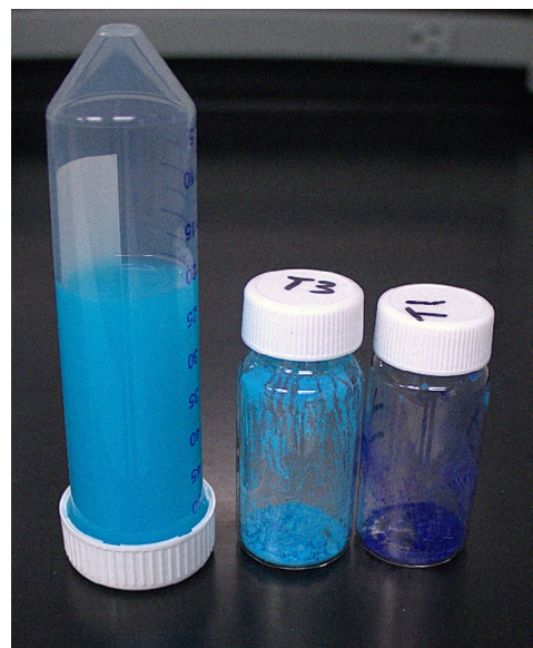
Figure 3. A digital image showing the various stages of the MOF preparation. After the 60 min incubation during the synthesis of carboxylate ligands with copper(II) ions a powder blue mixture was obtained. The partially dried MOFs retained a similar color after incubation at 100 °C (middle vial) which removed ethanol and some of the water. After incubation at 135 °C for 24 h, all water and DMF were removed resulting in dark navy blue-purple solid (right vial).
